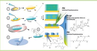
Schematic representation of membrane casting using a spin-coater. (a) Membrane fabrication procedure with (1) casting of the sacrificial layer, (2) casting of epoxy resin membrane material, (3) curing at 120 °C on a hotplate, (4) dissolution of pore templates and (5) final membrane release onto the water surface. (b) Representation of the microphase separation during the coating process and the final membrane with dissolved pore templates with indicated composition of the domains.
